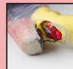
Cuts - core is visible -
