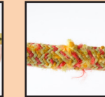
Slight damage to sheath
