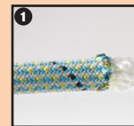
Sheath slippage - sheath is shorter -
