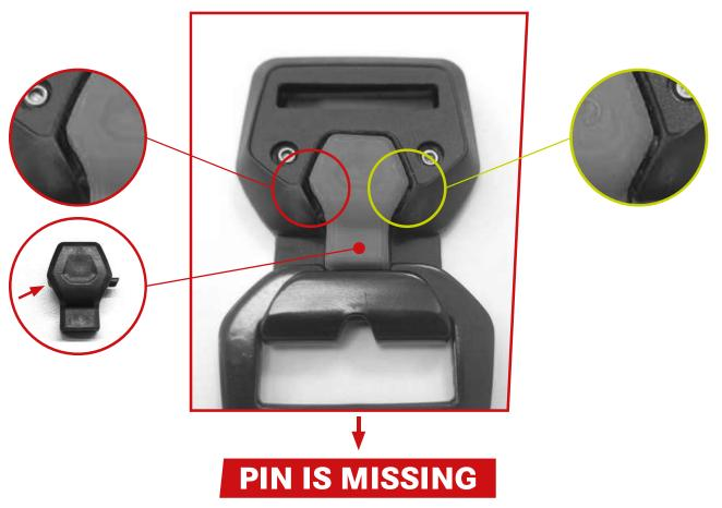
If a buckle is suspected to have a broken pin, this can be verified by applying slight pressure on the push button from behind using a tool like a Ballpoint pen, screwdriver or similar. If both pins are intact, the push button cannot be lifted out of the housing by applying slight pressure. If the pin is broken, the push button can be lifted out of the housing and a break will be visible.
